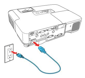
**Caution:** To avoid damaging the projector or lamp, never unplug the power cord when the power light is green or flashing orange.
